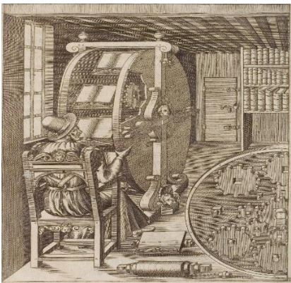
Ramelli’s “Book Wheel,” from The Various and Ingenious Machines of Captain Agostino Ramelli , 1588. Ramelli never actually built the device, but others did so, over the next two centuries, adapting Ramelli’s design for their own purposes.
